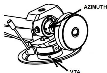
With the aid of a good magnifying glass adjust the needle until it is vertical in the groove (i.e. perpendicular to the record's surface). Ideally this should correspond to the top surface of the cartridge body being parallel to the record surface.
