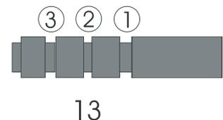
Hang the loop of the thread of the anti-skating weight in the groove of the anti-skating stub (13) corresponding to the downforce applied to your cartridge and feed the thread through the loop of the wire support (12).
